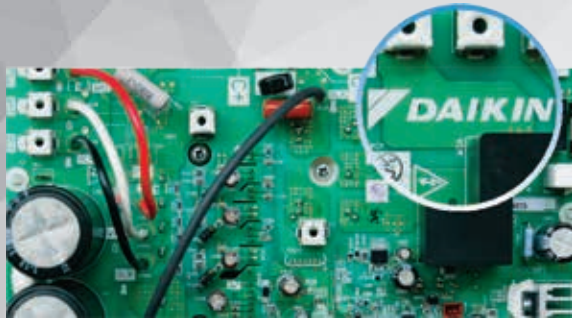
The inverter PCB of the compressor
